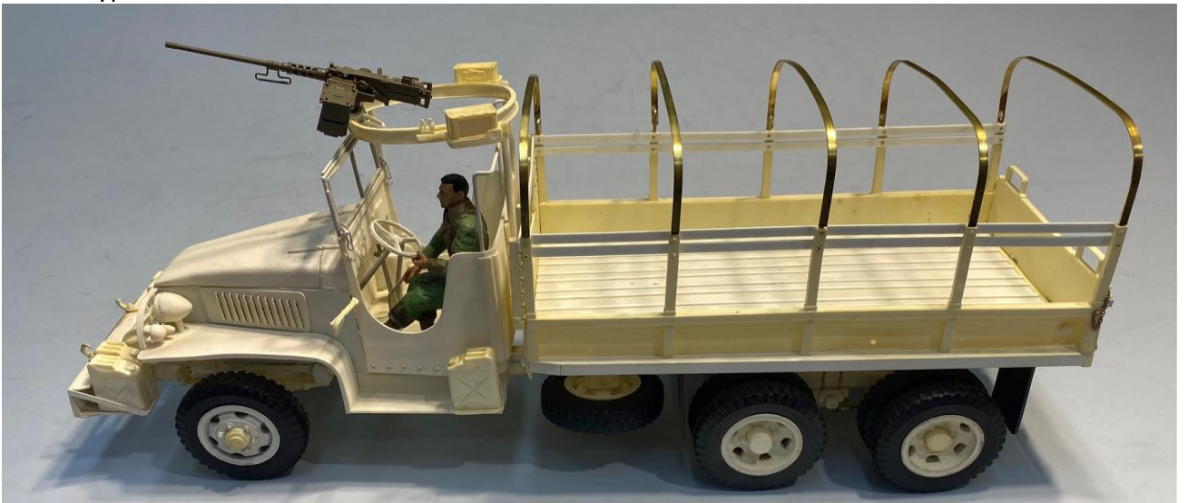
Truck #2: 2½ ton CCKW type 353 open cab, long cargo bed w/ canvass cover, dual rear axles and MG mount type M36
