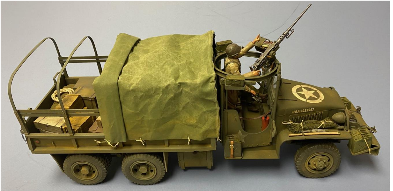
Truck #2: 2½ ton CCKW type 353 open cab, long cargo bed w/ canvass cover, dual rear axles and MG mount type M36
